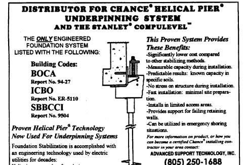
Helical screw anchor foundation system.
